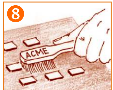
Clean board and pads with a brush and alcohol or acetone.
