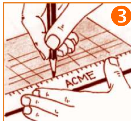
Draw footprints of each section and guidelines with pencil on the copper clad board. Planning ahead is important!
