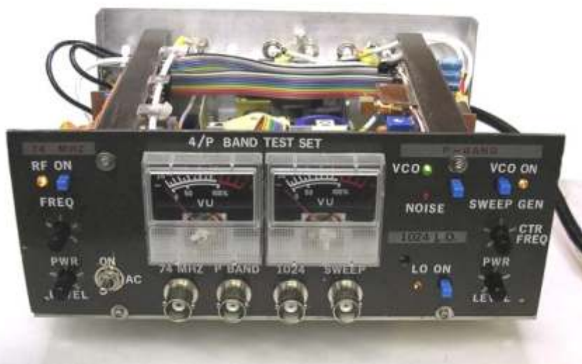
Fig. 23 – A Manhattan-built Test Set used to simulate three VHF receivers and contains a 1024 MHz Local Oscillator
