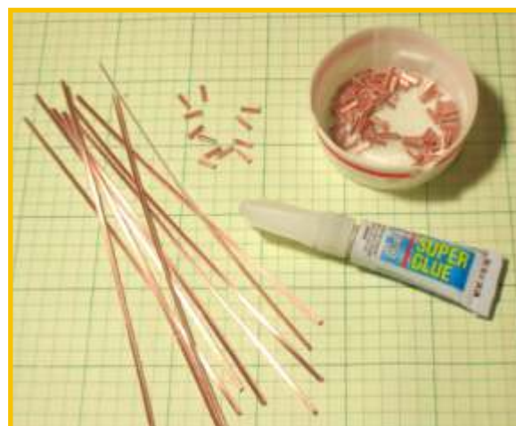
Fig. 3 – The basics for Manhattan-031. Strips of .031 copper clad are cut into narrow strips with a PCB shear or regular scissors; pads were made with a nibbling tool; super glue is used to affix the pads and strips to the main copper clad board.
