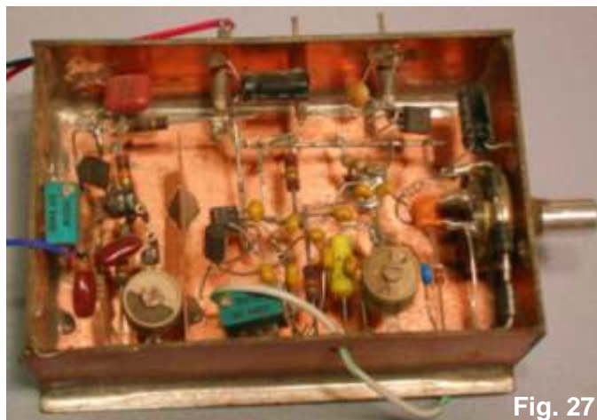
The modern “breadboard” is often a piece of copper clad. This 7.0 MHz VFO was built “ugly style” in a copper clad “box.”
