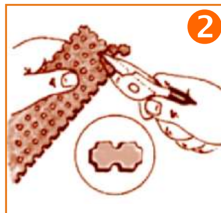
Using perforated copper clad circuit board for making the pads is another method, requiring no special tools.
