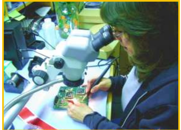
Fig. 8 – Connie Angel, one of the professional assemblers at the VLA observatory, solders surface mount components onto a board with tweezers and a soldering iron. The board is part of a new radio telescope (called ALMA) being built in Chile.
