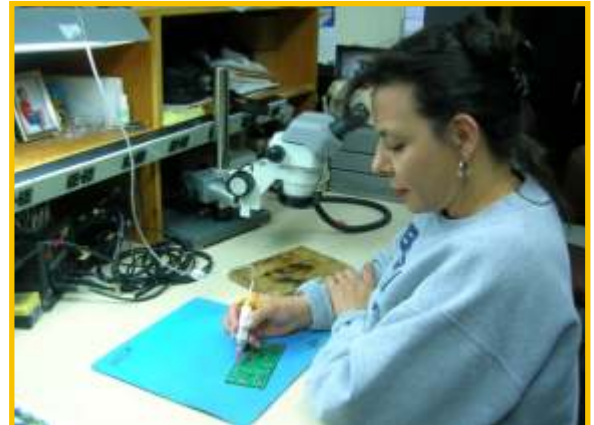
Fig. 21 – Professional assembler Mary Ellen Chavez applies solder paste to a PCB preparatory to reflow soldering.
