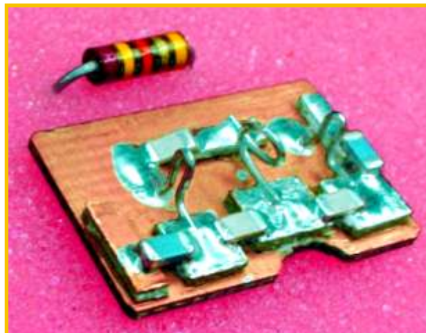
FIG. 16 – A 1090 MHz High Pass Filter made from SMC capacitors and “hand made” inductors Manhattan-031 style.
