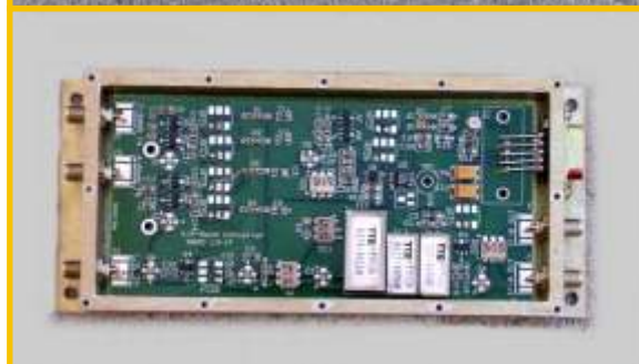
FIG. 19 – The Manhattan-031 prototype VHF upconverter (top) became the model for the PCB (bottom) with few differences, and mounted inside RFI enclosures.
