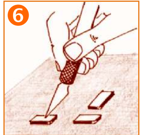
Place the pads onto the drop of glue and position with an Exacto knife, other sharp object or tweezers..
