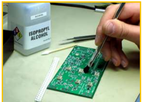
Fig. 9 – Clean solder connections with a hobby brush and alcohol. This keeps the board clean and free of corrosive rosin, whether building Manhattan or a PCB.
