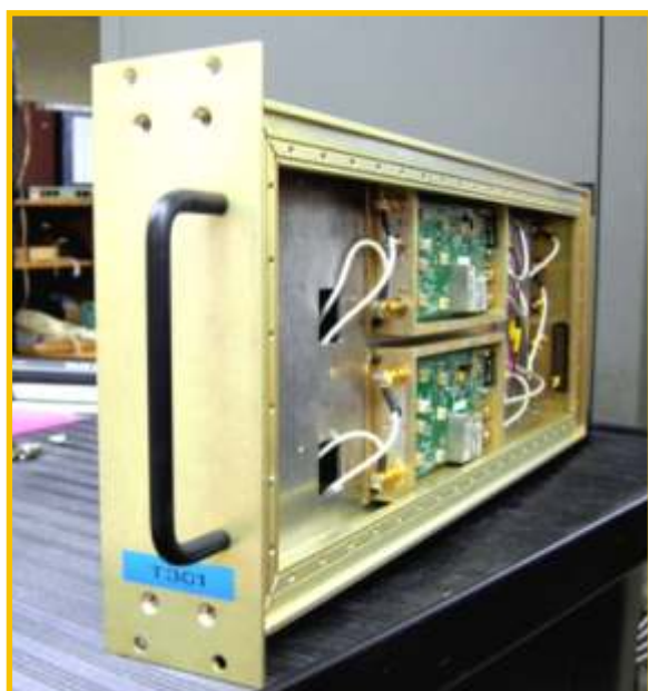
FIG. 20 – The finished VHF upconverter ready for installation in an antenna. There are two converters in each module, one for left-hand and right-hand polarization.
